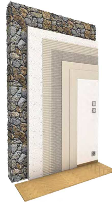
Wall-ACE external render in the old building as interior insulation
