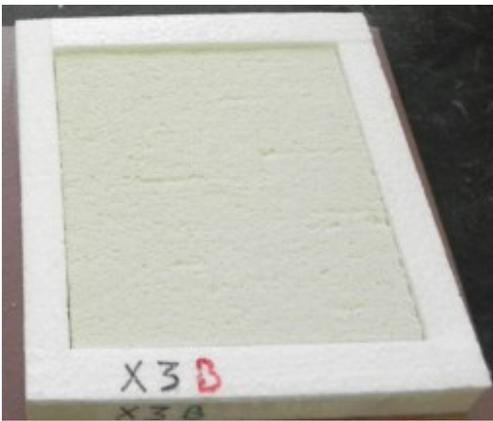
Figure 4: Typical sample of aerogel-based filling
