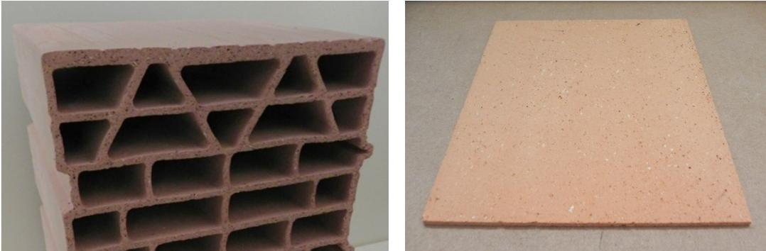
Figure 1: Section of hollow brick (left) and sample for testing of thermal conductivity on clay (right)
