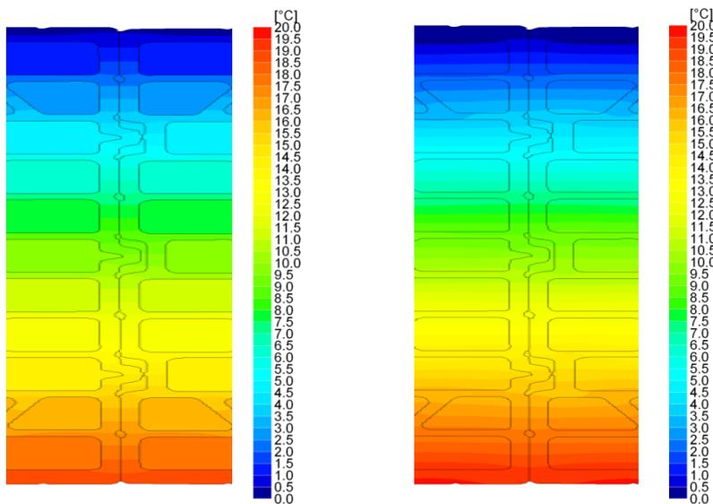
Figure 3: Sections of 2D temperature distribution for unfilled brick (left) and brick filled with mineral wool (right)
